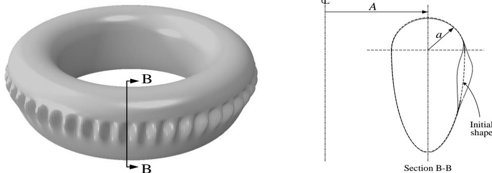
Figure 3: View of asymmetric bifurcation buckling mode for a tall toroid with  $b/a=3.0$ ,  $A/a=4$ ,  $a/t=200$ ,  $n=45$ ,  $p_{cr}=0.093MPa$
