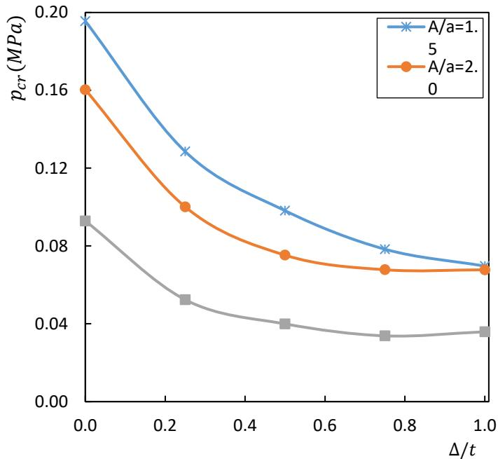
Figure 7: Sensitivity of critical buckling load to various amplitudes of first eigenmode imperfection in toroids with  $b/a = 3.0$ ,  $a/t = 200$  and different  $A/a$  ratios
