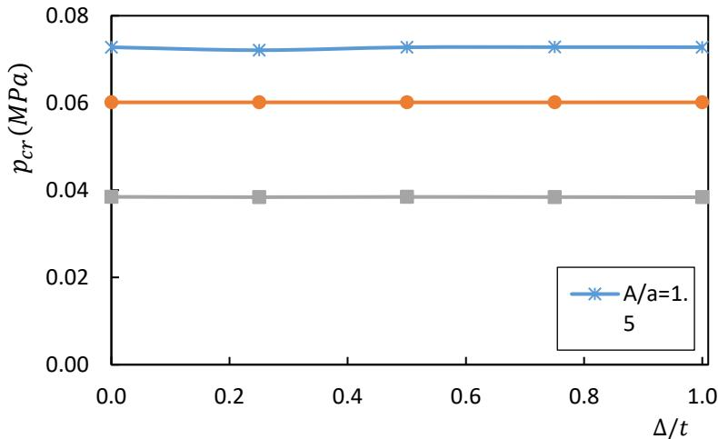
Figure 9: Sensitivity of critical buckling load to various amplitudes of first eigenmode imperfection in toroids with  $b/a = 0.5$ ,  $a/t = 200$  and different  $A/a$  ratios
