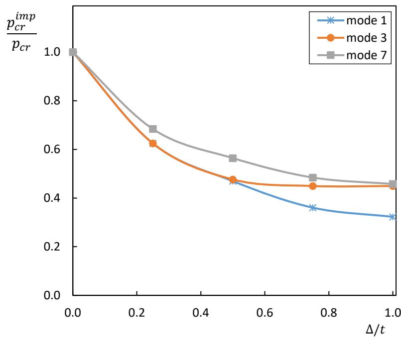
Figure 6: Effect of imperfection amplitude of various eigenmodes on the buckling pressures of toroids with  $b/a = 3.0$ ,  $A/a = 2.0$ ,  $a/t = 200$
