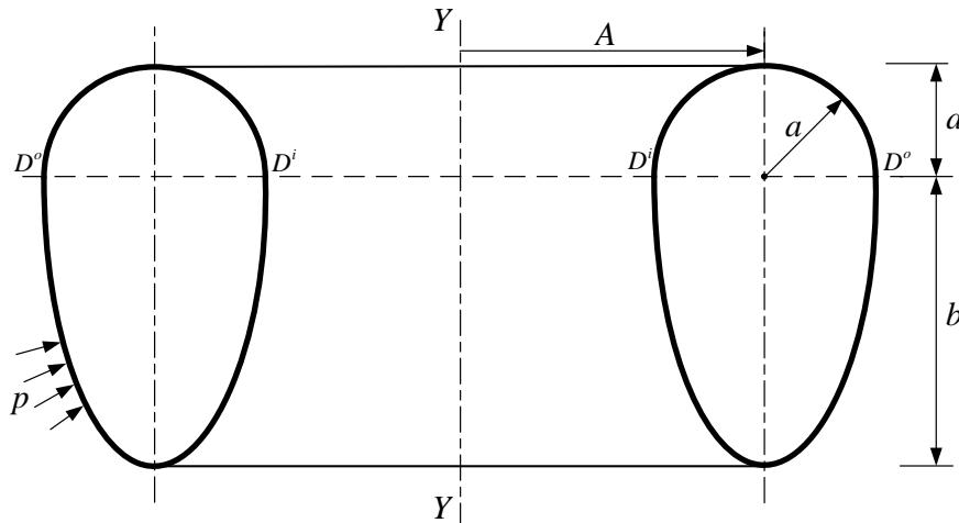
Figure 2: Externally pressurised circular-elliptic toroidal vessel
