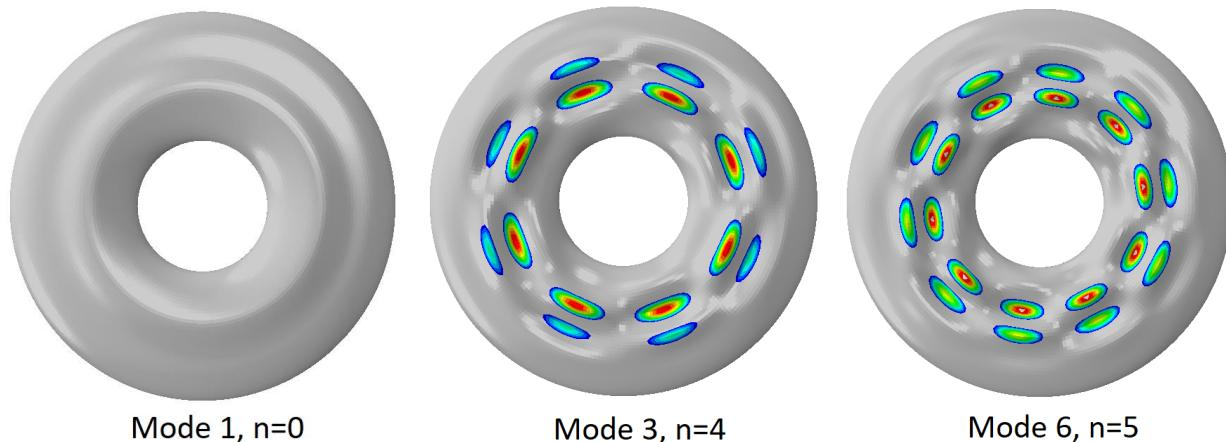
Figure 4: Bottom view of eigenmode of a *short* circular-elliptic toroid with  $b/a = 0.5$ ,  $A/a = 2.0$ ,  $a/t = 200$
