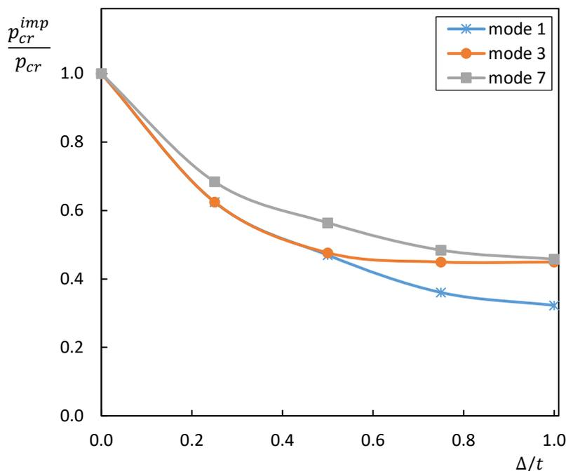
Figure 6: Effect of imperfection amplitude of various eigenmodes on the buckling pressures of toroids with  $b/a = 3.0$ ,  $A/a = 2.0$ ,  $a/t = 200$
