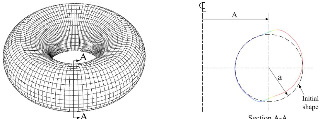
Figure 5: View of axisymmetric bifurcation buckling mode for a short toroid with  $b/a = 1$ ,  $A/a = 2$ ,  $a/t = 200$ ,  $n = 0$ ,  $p_{cr} = 0.108 \text{ MPa}$
