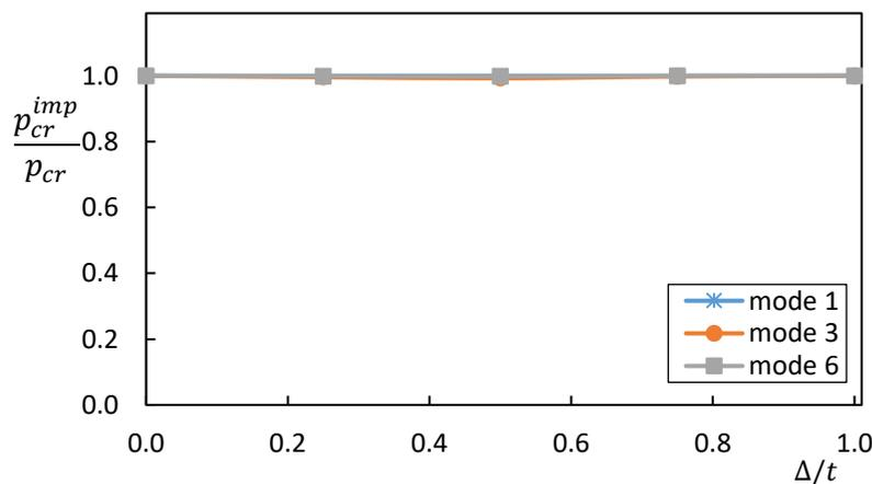
Figure 8: Effect of imperfection amplitude of various eigenmodes on the buckling pressures of toroids with  $b/a=0.5$ ,  $A/a=2.0$ ,  $a/t=200$
