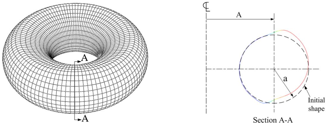
Figure 5: View of axisymmetric bifurcation buckling mode for a short toroid with  $b/a=1$ ,  $A/a=2$ ,  $a/t=200$ ,  $n=0$ ,  $p_{cr}=0.108MPa$
