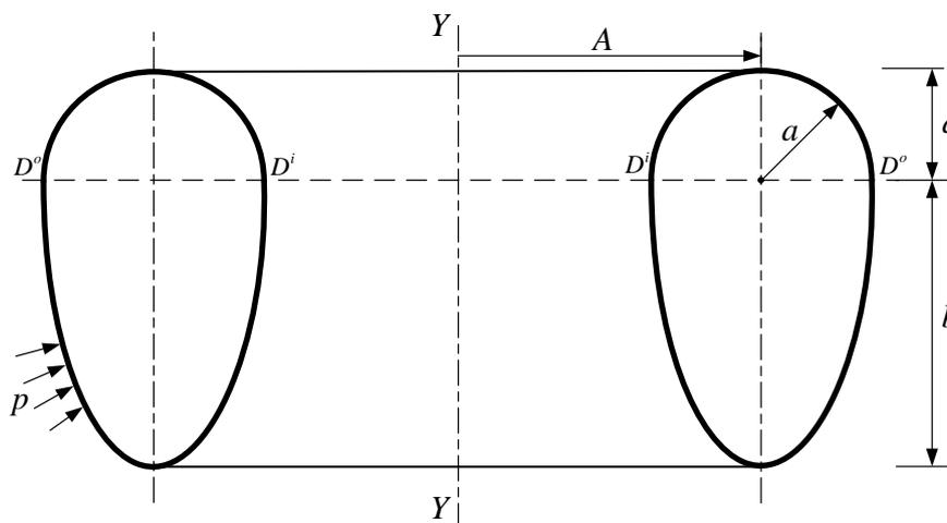
Figure 2: Externally pressurised circular-elliptic toroidal vessel
