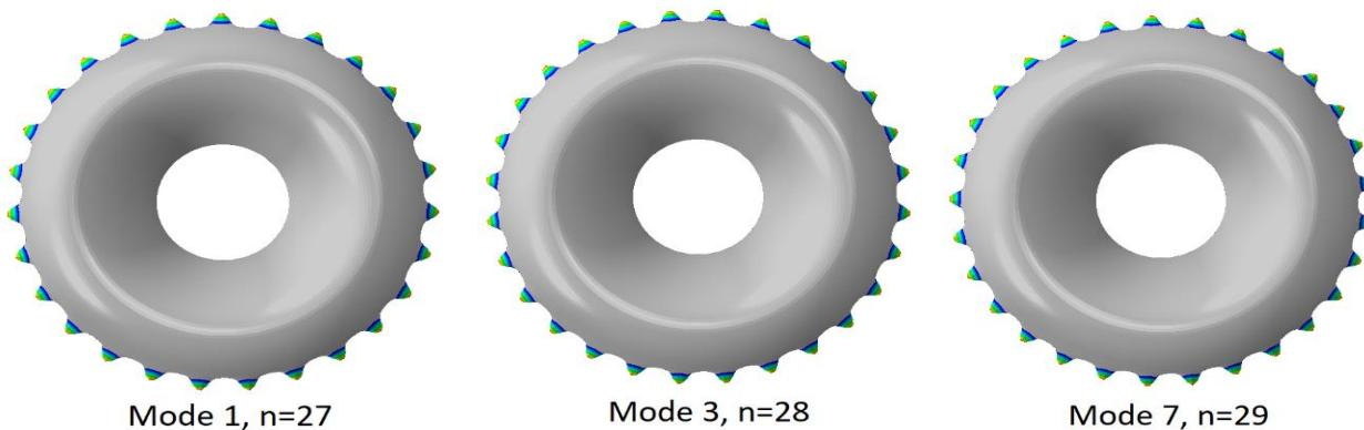
Figure 2: Bottom views of eigenmodes of a *tall* circular-elliptic toroid with  $b/a=3.0$ ,  $A/a=2.0$ ,  $a/t=200$
