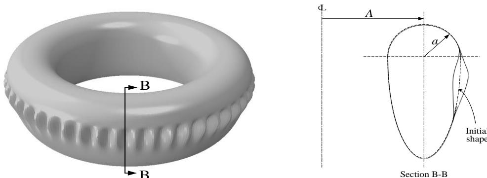
Figure 3: View of asymmetric bifurcation buckling mode for a tall toroid with  $b/a=3.0$ ,  $A/a=4$ ,  $a/t=200$ ,  $n=45$ ,  $p_{cr}=0.093\text{MPa}$
