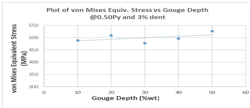
**Figure 8: Effect of gouge depth on von Mises Equivalent stress at 3% OD dent**
