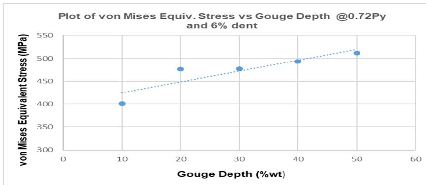
**Figure 9: Effect of gouge depth on von Mises Equivalent stress at 6% OD dent**
