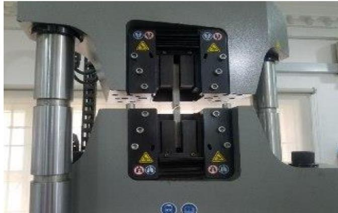
**Figure 2: Ruptured tensile test Specimen**
