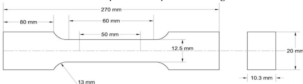
**Figure 1: Rectangular tension test specimen**
