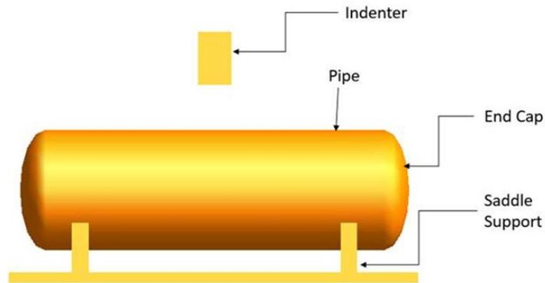
**Figure 4: Test set up of Indenter and Pipe**
