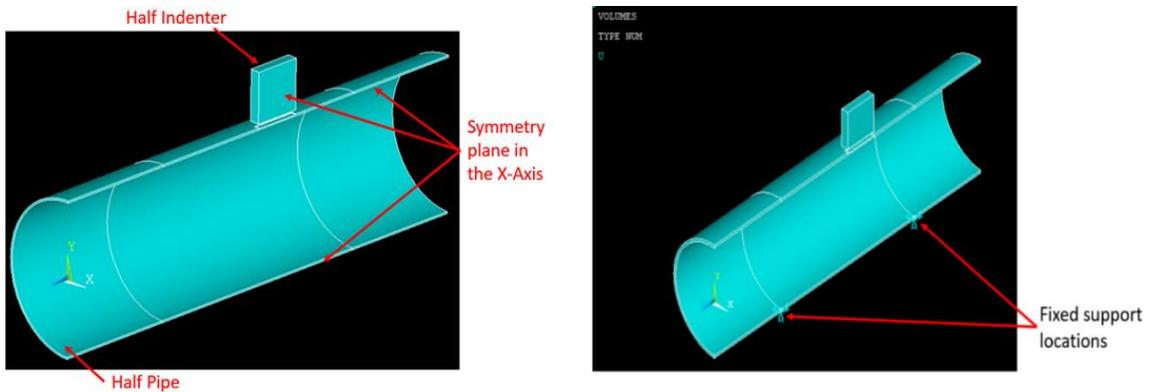
**(a) Pipe & indenter modelled with symmetry planes (b) Model showing anchor support locations**
