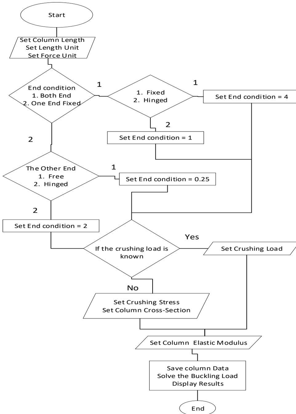
Figure 3: Flow Chart used for Column Design
