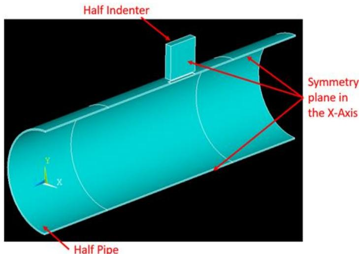
Figure 4: Half pipe model with symmetry planes and support locations
