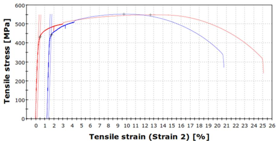
Figure 2: Stress-strain curves for API 5L X52 pipe
