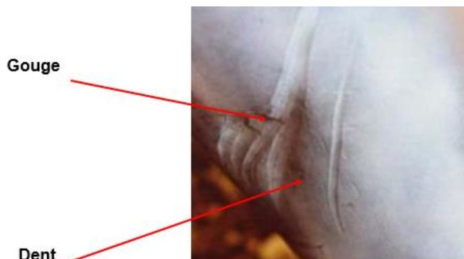
Figure 1: Pictorial presentation of the combined dent and gouge defect [5]
