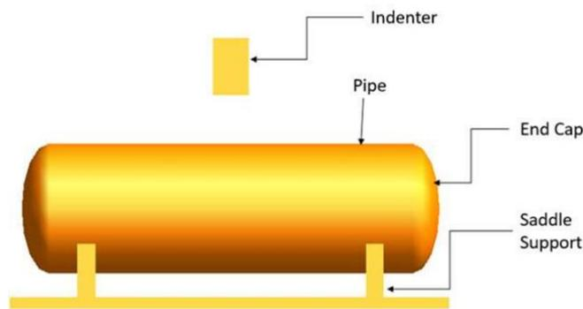
Figure 3: Test set up of Indenter and Pipe
