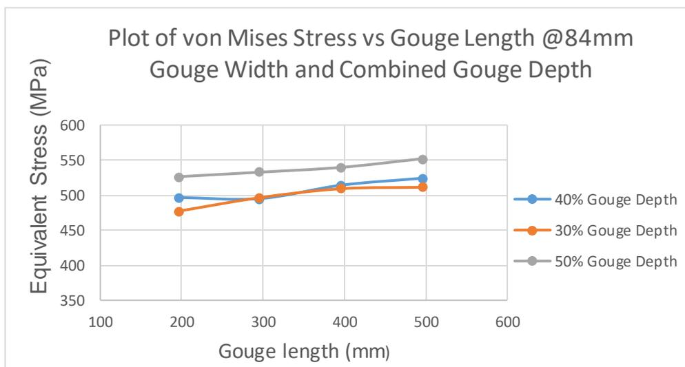
Figure 6: Plot of von Mises Stress vs Gouge Length @84mm Gouge Width and Combined Gouge Depth
