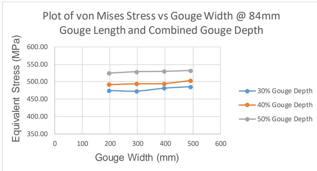
Figure 7: Plot of von Mises Stress vs Gouge Width @ 84mm Gouge Length and Combined Gouge Depth
