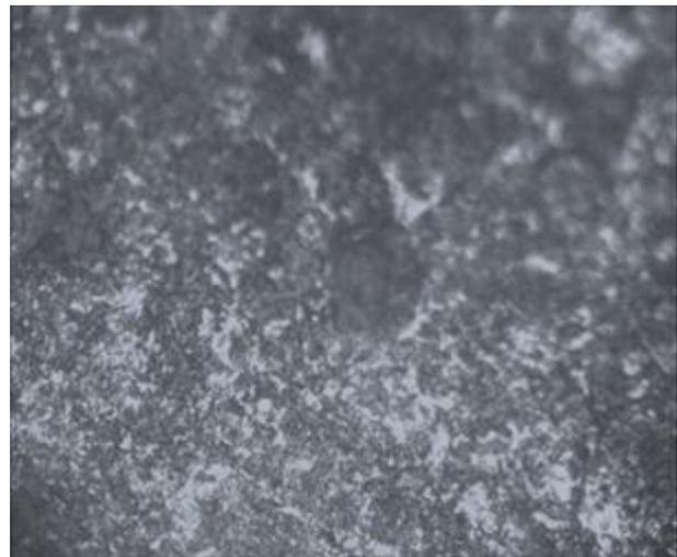
Plate 1b: Optical Micrograph of Austempered 0.3% C Steel at 300°C Immersed in Sea Water for 15 Days - (200X)
