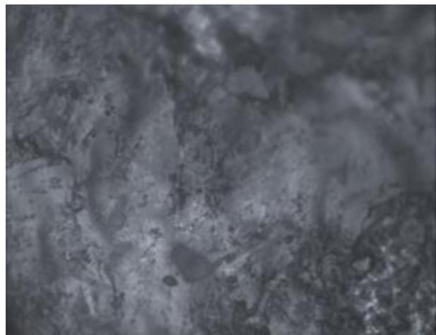
Plate 5d: Optical Micrograph of Austempered 0.3%C Steel at 340°C Immersed in Sea Water 75 Days - (200X)
