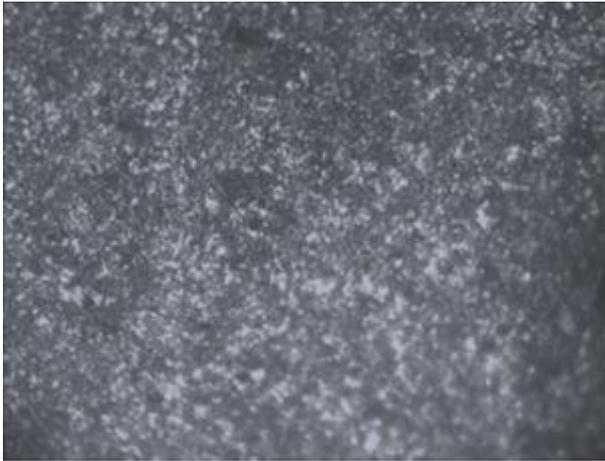
Plate 1c: Optical Micrograph of Austempered 0.3% C Steel at 320°C Immersed in Sea Water for 15 Days - (200X)
