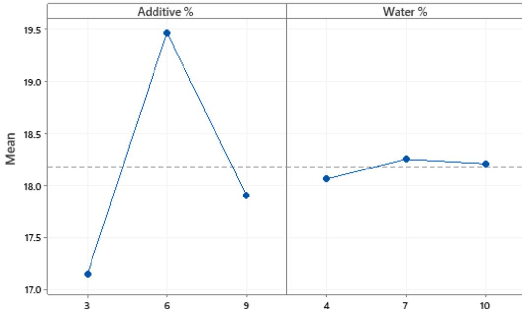
**Figure 2: Main Effects Plots of Green Shear Strength (GSS)**
