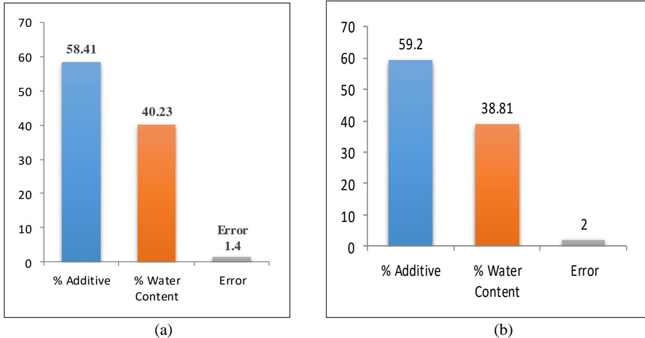
**Figure 3: Charts showing the relative contribution of Gelatine Cassava Additive on the Green Compressive Strength (a) and Green Shear strengths (b) of Bida Moulding Sand**
