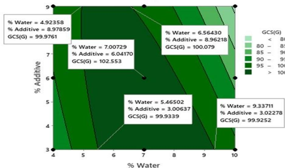
Figure 4: Contour plots of a Response (GCS) vs. % Additive and % Water Content
