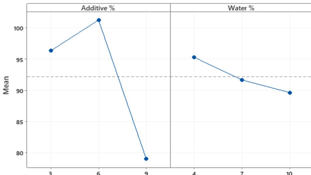
Figure 1: Main Effects Plots of Green Compressive Strength (GCS)
