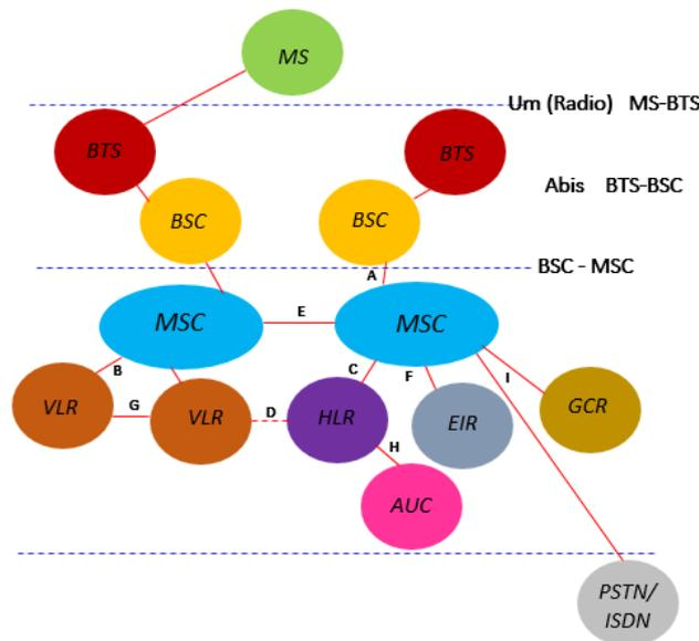
Figure 3. MAP Interfaces on GSM Network
