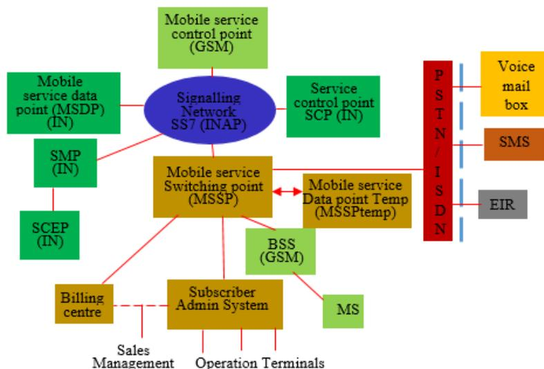
Figure 5. Block Diagram of GSM-IN integration Architecture
