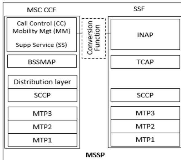
**Figure 6. Signaling protocol stack for MSSP illustrating the interacting between the SSP and the MSC**
