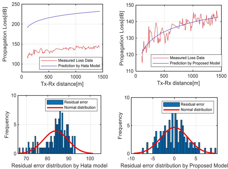
Fig 3: Measured propagation loss estimation using the original  $PL_{COST-234}$  and the proposed adapted  $PL_{COST-234}$  for Cell\_3
