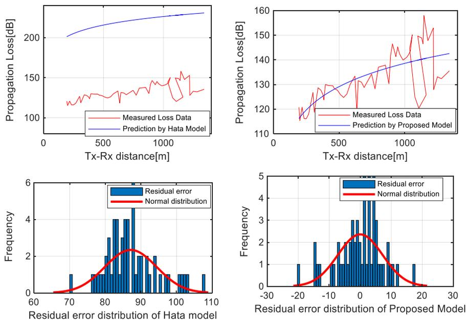
Fig 2: Measured propagation loss estimation using the original  $PL_{COST-234}$  and the proposed adapted  $PL_{COST-234}$  for Cell\_2
