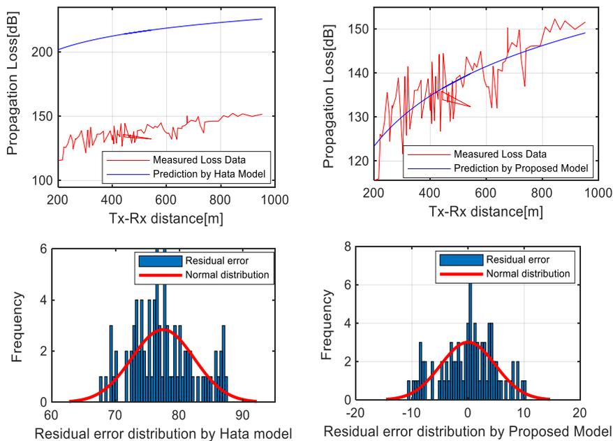
Fig 4: Measured propagation loss estimation using the original  $PL_{COST-234}$  and the proposed adapted  $PL_{COST-234}$  for Cell\_4
