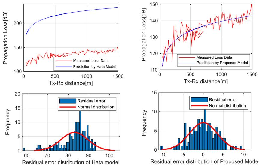
Fig 1: Measured propagation loss estimation using the original  $PL_{COST-234}$  and the proposed adapted  $PL_{COST-234}$  for Cell\_1
