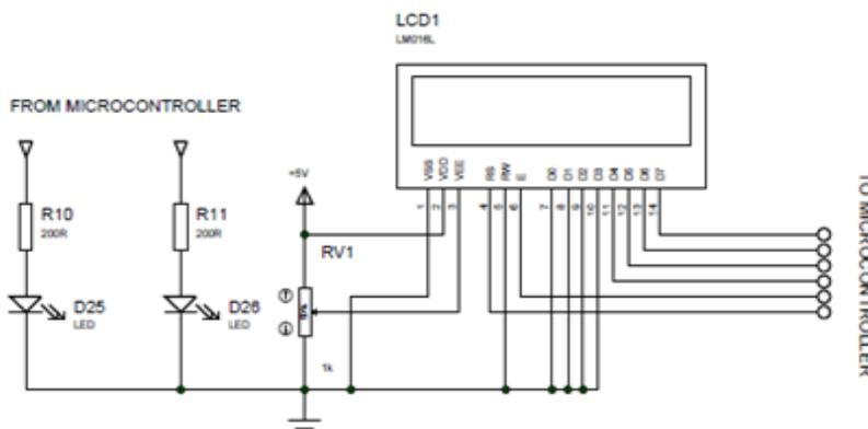
Figure 8: Display Circuit
