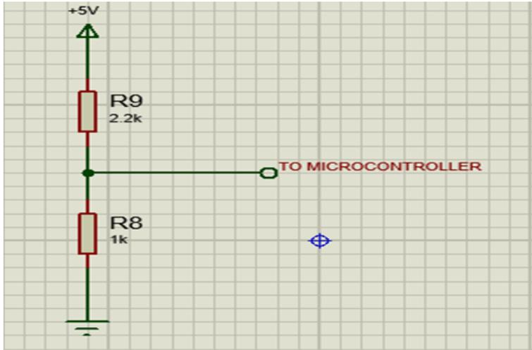
Figure 4: Battery Voltage Sensor unit
