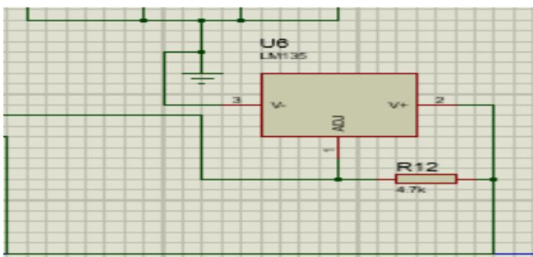
Fig. 10: Temperature Sensor Circuit
