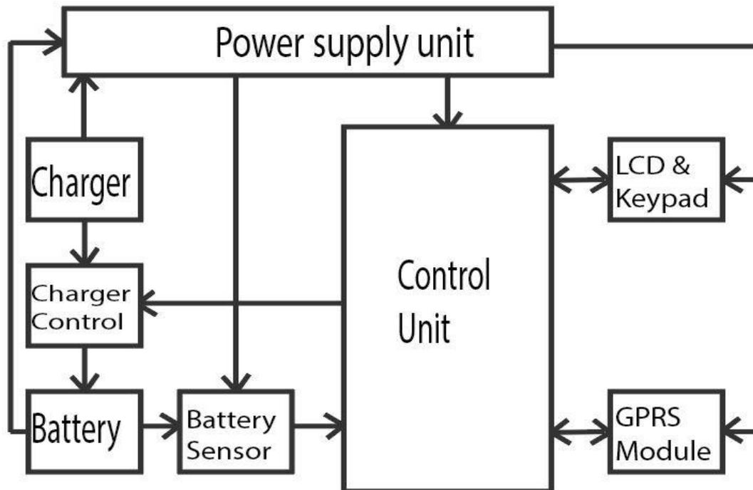
Figure 1: Block Diagram of the Battery Charging, Monitoring & Control Device
