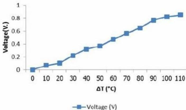
Figure 9: Graph the relationship between Voltage and Temperature Difference.
