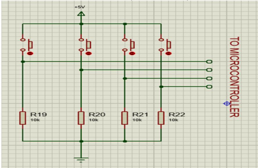
Figure 7: Button Circuit
