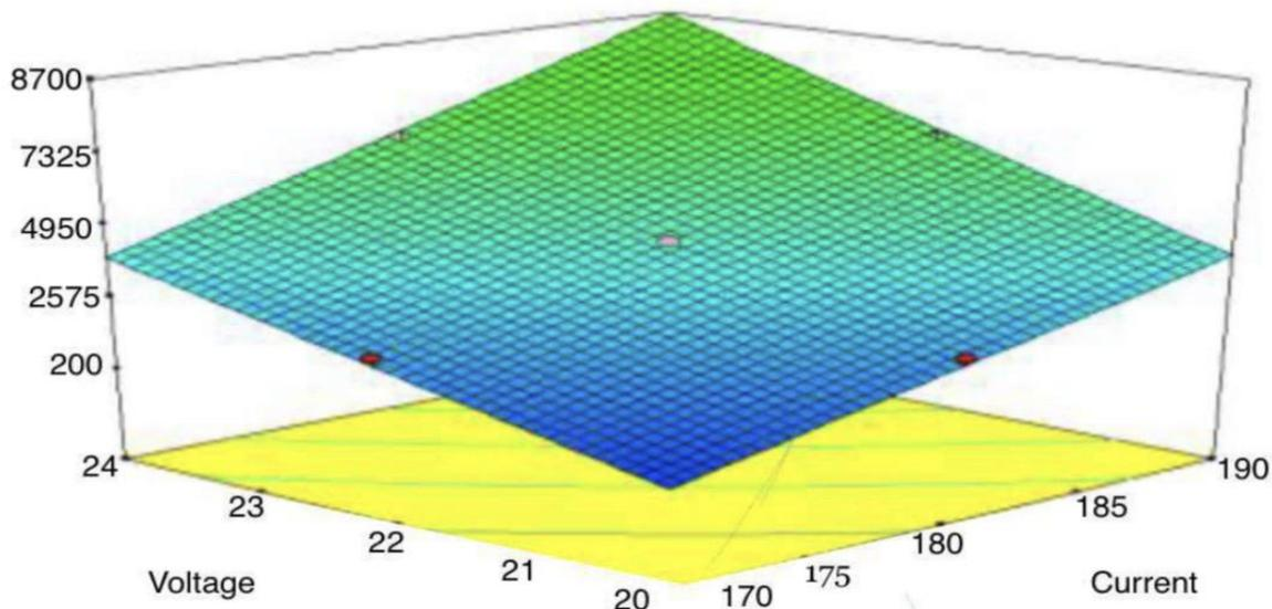
Figure 2 shows the effects of voltage and current on heat input
