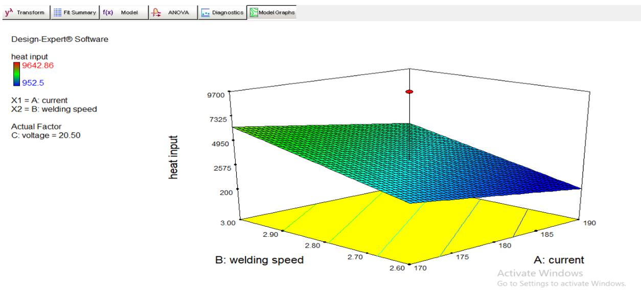
Figure 1: Effect of Welding speed and Current on Heat Input
