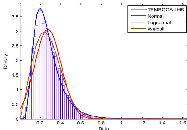
Figure 2: Probability Density Frequency of FoS of the gully wall LHS slope stability
