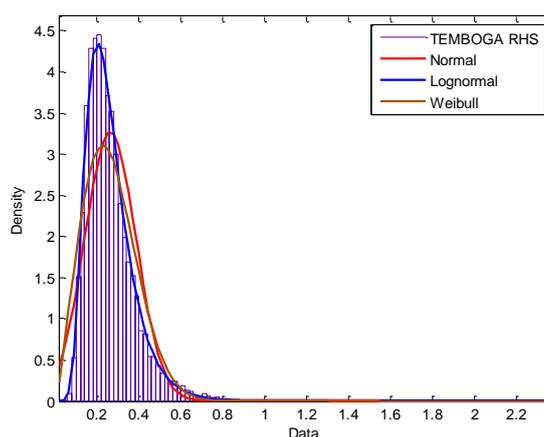
Figure 3: Probability Density Frequency of FoS of the gully wall RHS slope stability
