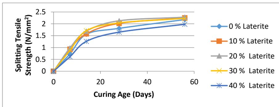
Figure 7: Splitting Tensile Strength of Laterized Concrete with curing age.
