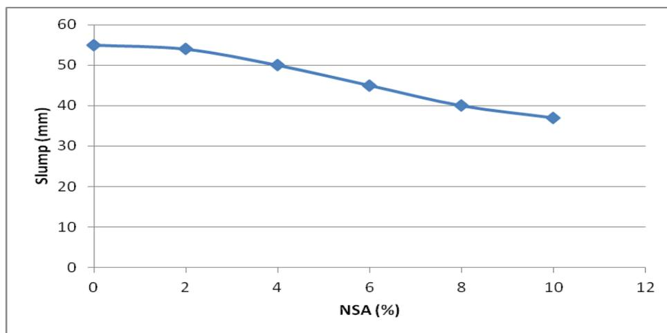
Figure 5: Slump of NSHA-Concrete at optimum laterite content of 20 %
