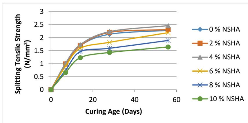
Figure 9: Splitting Tensile Strength of NSHA-Concrete with curing age at optimum Laterite Content of 20 %
