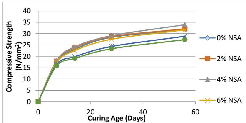
Figure 8: Compressive Strength of NSHA-Concrete with curing age at optimum Laterite Content of 20 %
