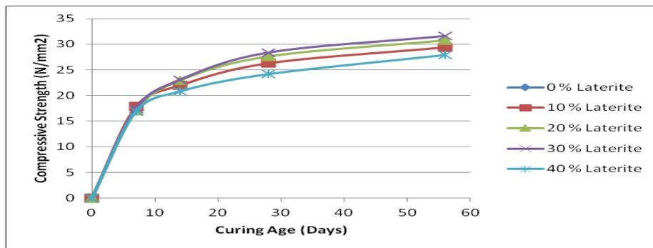
Figure 6: Compressive Strength of Laterized Concrete with curing age in days.
