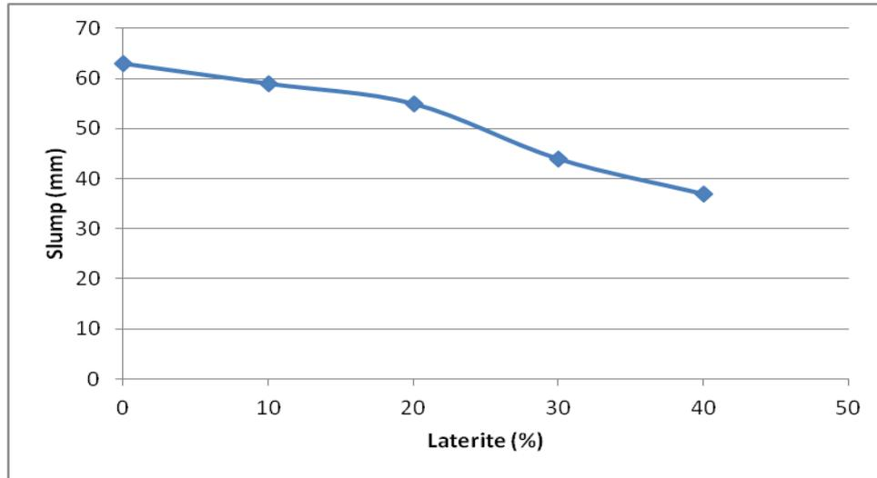
Figure 4: Slump of Laterized Concrete
