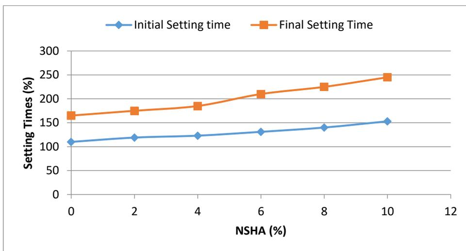
Figure 3: Initial and final setting time of NSHA-Cement Paste
