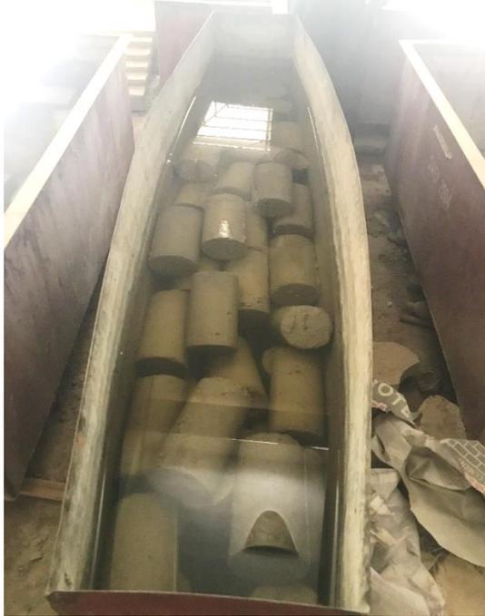
Plate 2: Curing of concrete specimens
