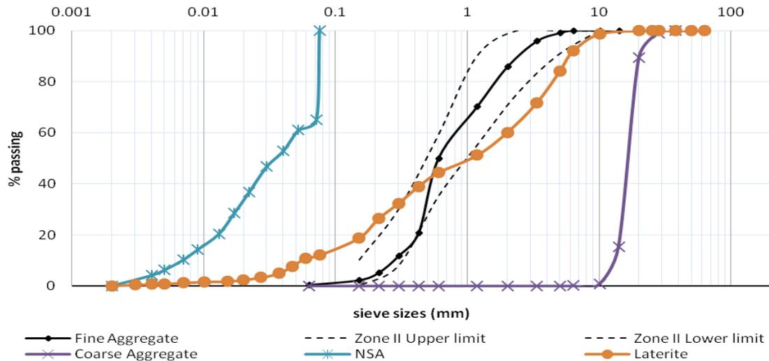
Figure 1. Particle Size Distribution of Fine Aggregate, Granite, Laterite and NSHA
