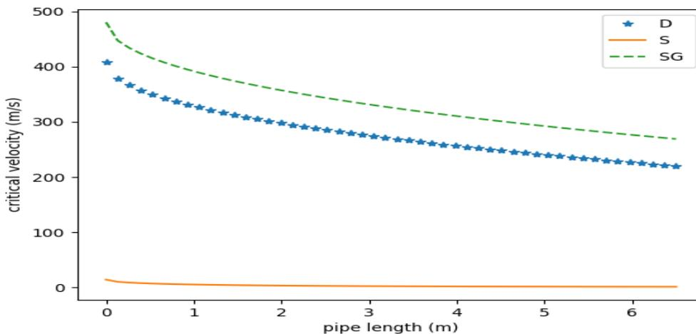
**Figure 8: Critical velocity profiles as a function of pipe length reflecting the effect of the three flow patterns: stratified, slug and dispersed bubble flow with three cases of initial fluid mixture velocity (0.2m/s 0.4m/s 0.8m/s),  $d_p=320 \mu\text{m}$  and  $p_d = 0.5\text{m}$**
