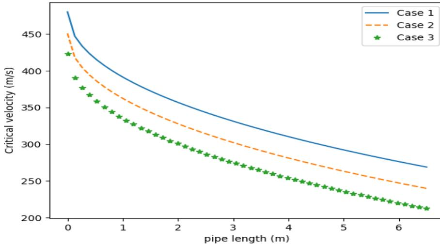
**Figure 4:** Critical velocity profile as a function of pipe length with fluid mixture velocity 0.2m/s, 0.4m/s, 0.8m/s  $d_p=320 \mu\text{m}$ , and  $p_d = 0.5\text{m}$  for slug flow operating conditions.
