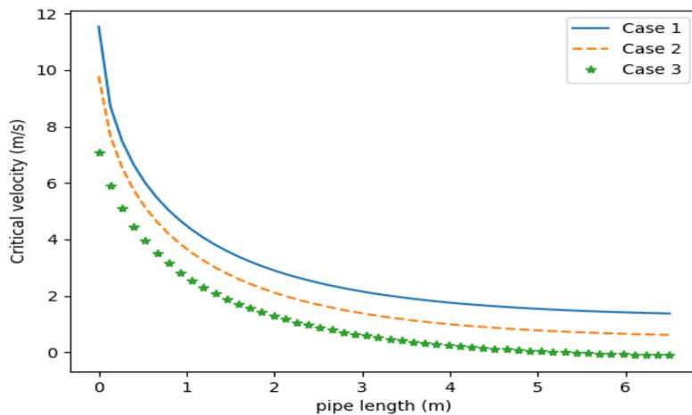
**Figure 3: Critical velocity profile as a function of pipe length with fluid mixture velocity (1.0m/s, 2m/s, 4.m/s)  $d_p=320 \mu\text{m}$ , and  $p_d = 0.5\text{m}$  for stratified flow operating conditions**
