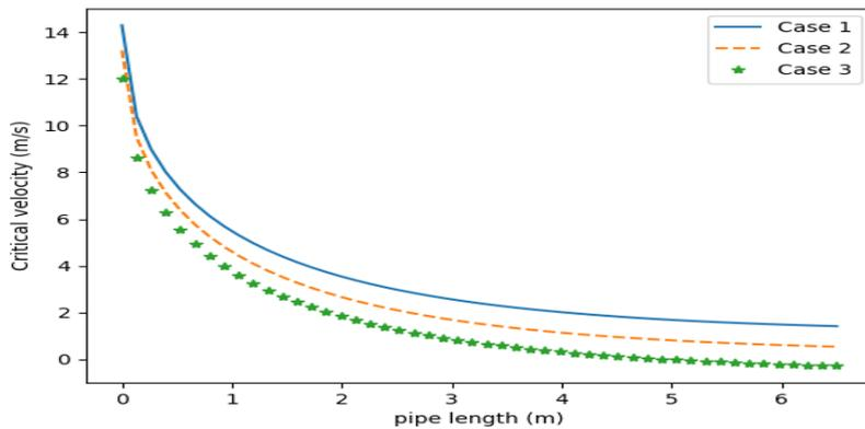
**Figure 2: Critical velocity profile as a function of pipe length with fluid mixture velocity (0.2m/s, 0.4m/s, 0.8m/s)  $d_p=320 \mu\text{m}$ , and  $p_d = 0.5\text{m}$  for stratified flow operating conditions**
