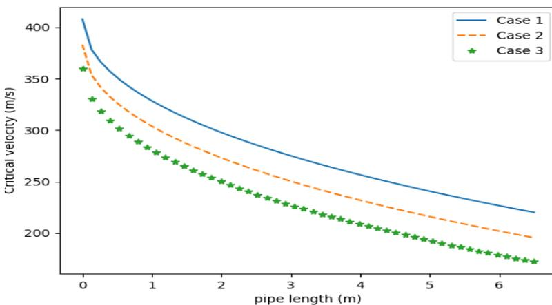
**Figure 6:** Critical velocity profile as a function of pipe length with fluid mixture velocity 0.2m/s, 0.4m/s, 0.8m/s  $d_p=320 \mu\text{m}$ , and  $p_d = 0.5\text{m}$  for dispersed bubble flow operating condition
