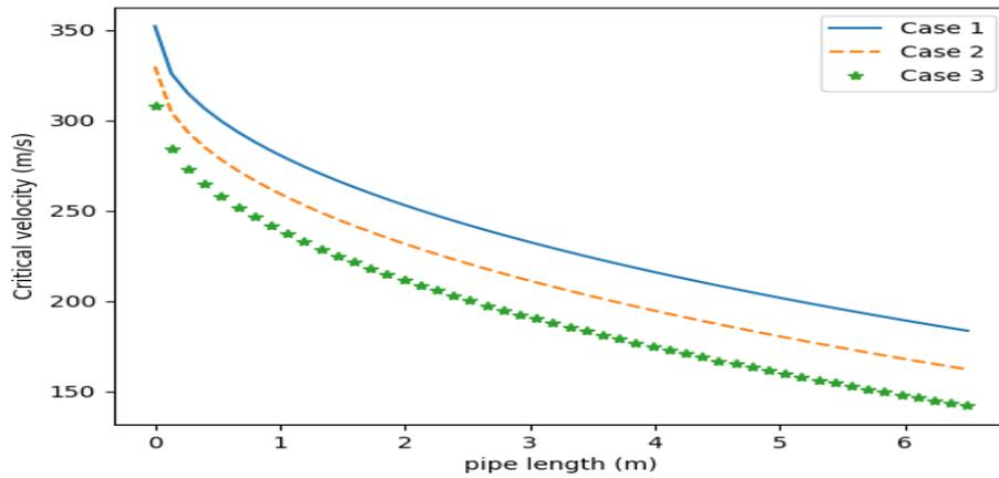
**Figure 7: Critical velocity profile as a function of pipe length with fluid mixture velocity 1.0m/s, 2m/s, 4m/s  $d_p=320 \mu\text{m}$ , and  $p_d = 0.5\text{m}$  for dispersed bubble flow operating conditions**
