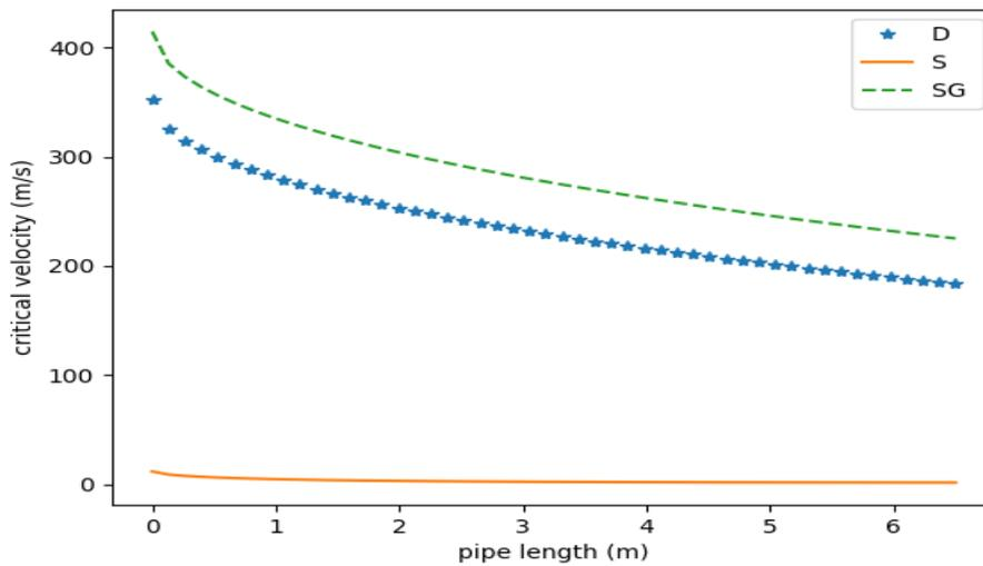
**Figure 9: Critical velocity profiles as a function of pipe length reflecting the effect of the three flow patterns: stratified, slug and dispersed bubble flow with three cases of initial fluid mixture velocity (1.0m/s 2.0m/s 4.0m/s),  $d_p=320 \mu\text{m}$  and  $p_d = 0.5\text{m}$**
