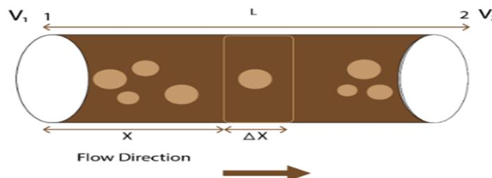
**Figure 2: Pictorial View of Multiphase Fluids Flow in a Horizontal Pipeline**
