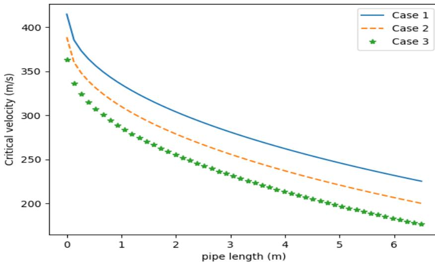
**Figure 5:** Critical velocity profile as a function of pipe length with fluid mixture velocity 1.0m/s, 2m/s, 4m/s  $d_p=320 \mu\text{m}$ , and  $p_d = 0.5\text{m}$  for slug flow operating conditions
